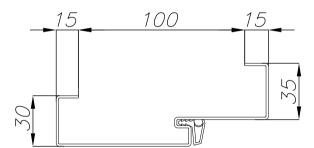
Adjustable metal door frame (only the rebated system) made of 1.5 mm thick sheet steel, available with standard powder coatings in the following colours: white (RAL 9016), grey (RAL 7040), brown (RAL 8017) and beige (RAL 1001). Door frames painted in non-standard colours from RAL or NCS systems are available upon consultation with the Sales Department. The door frame consists of a major part and an architrave inserted into the major part.
