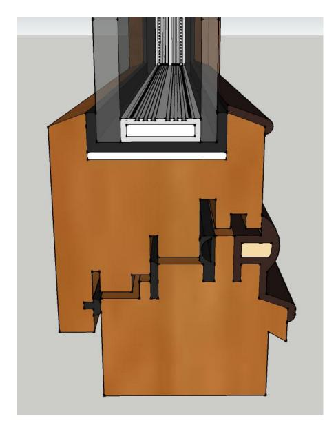
Soundproof window showing the 3 seals and glazing with wide air-gap and panes of different thicknesses
