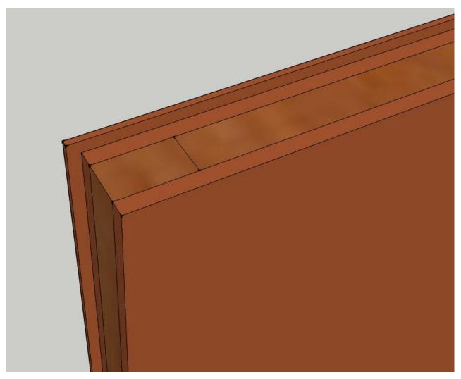
Soundproof door leaf showing internal frame, front and rear HDF faces, and rebate machined out of the front HDF face
