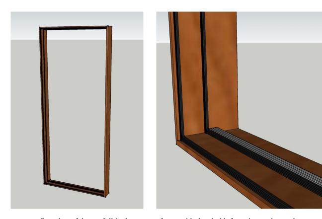
Soundproof door – full-lock aperture frame with threshold, featuring gasket seals for the front door rebate and the rear face perimiter.
