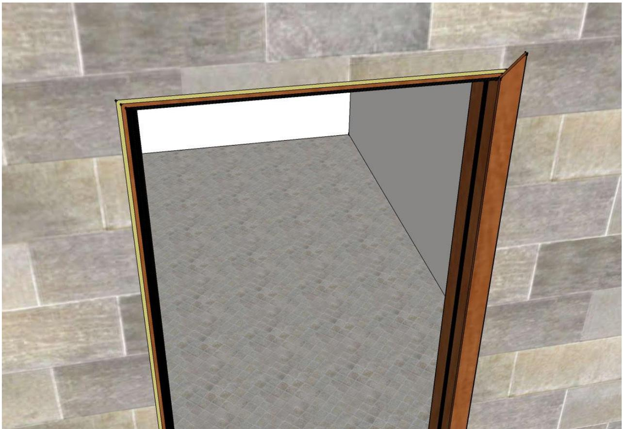
Installed aperture frame showing expandible foam sealing the gap between the aperture and the wall, and part of the aesthetic frame
