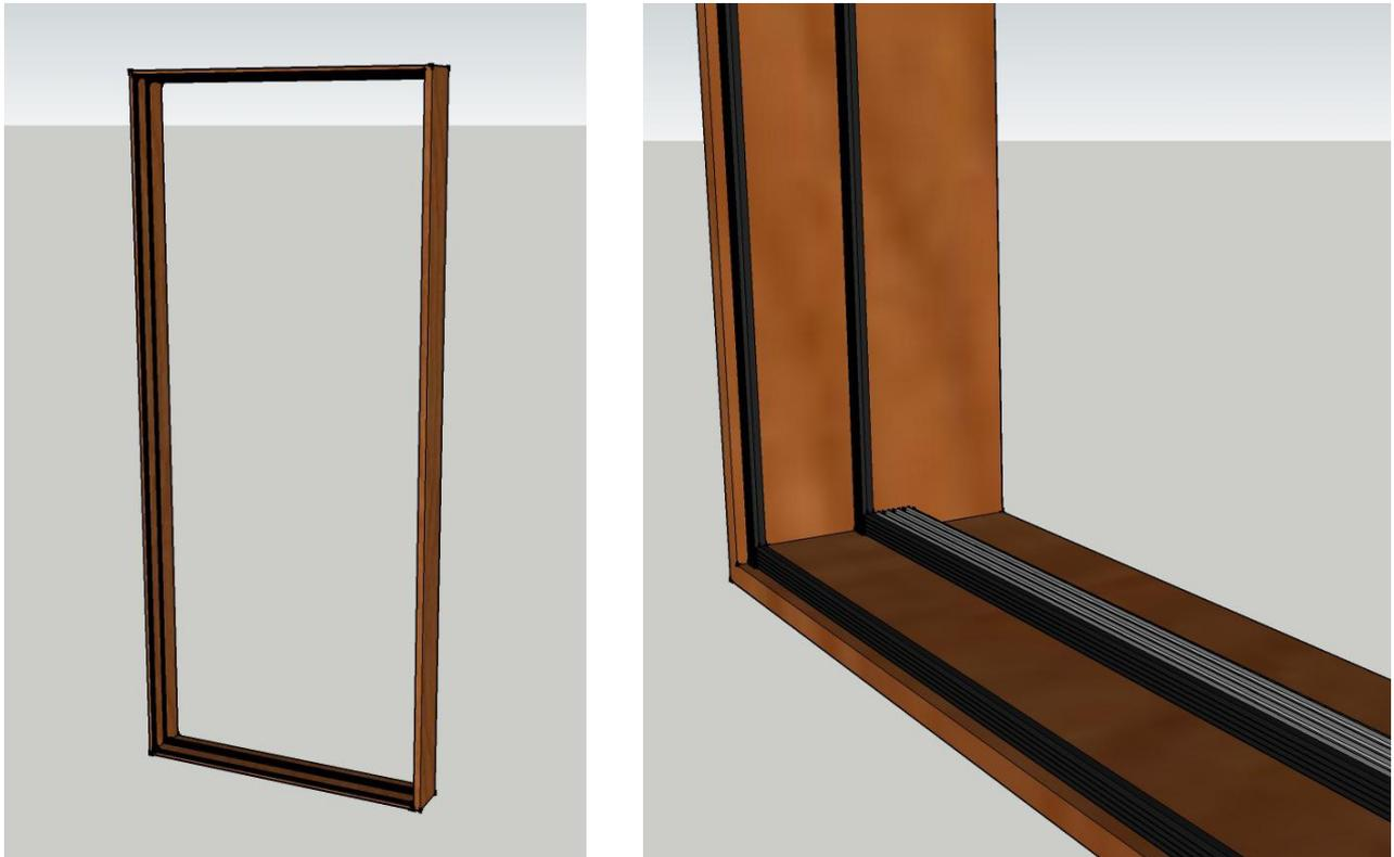
Soundproof door – full-lock aperture frame with threshold, featuring gasket seals for the front door rebate and the rear face perimeter.
